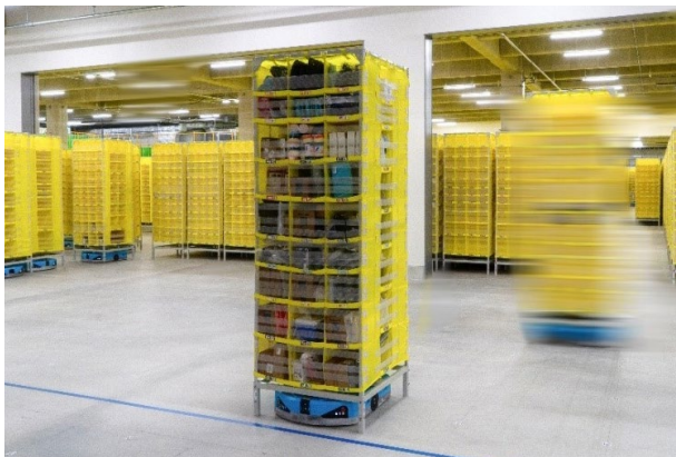
Amazon Robotics conveys shelves of products to the packaging stations, reducing the time it takes to pick such items from shelved inventories.
